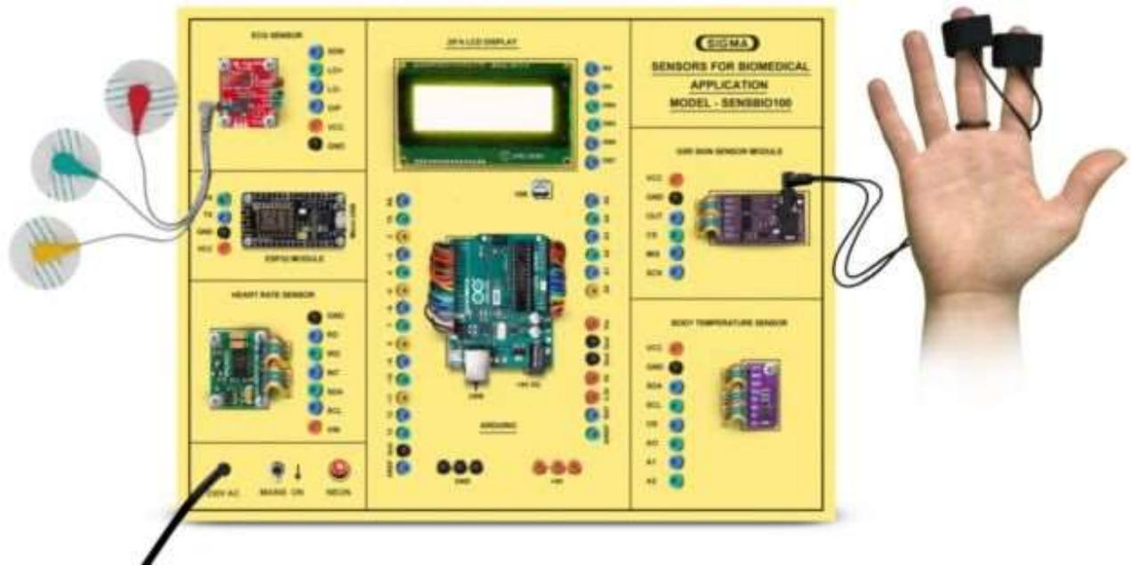
This trainer has been designed with a view to provide practical and experimental knowledge of Biomedical Sensors programming for Internet of Things (IOT) with Arduino IOT Board.
